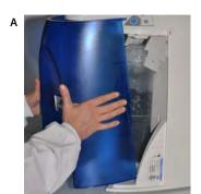
• Open the front cover (this may require to remove the final filter) to go into STANDBY mode (A).
