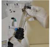
• Carefully insert the UV Lamp into the UV housing (G).
