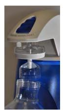
Measure the total volume of water (in Litres) dispensed from the system using a 1 L graduated cylinder.
